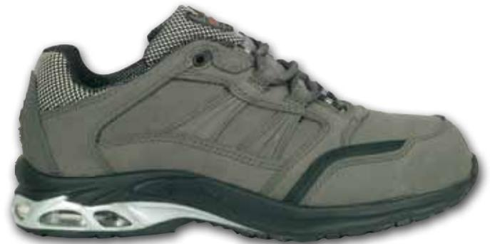
**RED EYE S3****36-48****TOMAIA:** nubuck idrorepellente**FODERA:** tessuto traspirante, assorbente e deassorbente, antiabrasione**SOLETTA:** intera, anatomica, forata, estraibile, antistatica, rivestita in tessuto**SUOLA:** PU/Gomma nitrilica**PUNTALE:** acciaio**LAMINA:** non metallica APT Plate**CALZATA:** 11 Mondopoint
